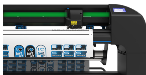
GREEN status = Working
