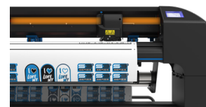
ORANGE status = Lift pinch rollers
